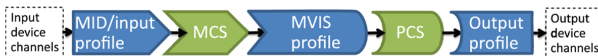
Figure 3 — Workflow connecting a MultiplexIdentification (MID)/input profile, a MultiplexVisualization (MVIS) profile and an output profile
