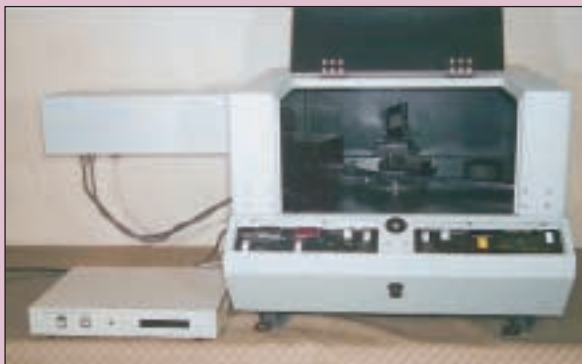
Figure 4. Instruments used for physical analysis of light reflection and transmission. The goniophotometer (left) measures light scatter as a function of variable angles of illumination or observation. This instrument is useful for studies of gloss, luster, surface smoothness (or roughness), haze, and distinctness of image. A spectrophotometer measures and analyzes the reflected light from a surface wavelength by wavelength as a means of determining the color of that surface. The unit shown here (right) is an automated scanning spectrophotometer that measures both reflected and transmitted light. Handheld spectrophotometers about the size of densitometers are also available.
