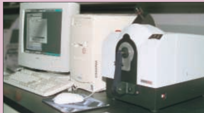
Figure 4. Instruments used for physical analysis of light reflection and transmission. The goniophotometer (left) measures light scatter as a function of variable angles of illumination or observation. This instrument is useful for studies of gloss, luster, surface smoothness (or roughness), haze, and distinctness of image. A spectrophotometer measures and analyzes the reflected light from a surface wavelength by wavelength as a means of determining the color of that surface. The unit shown here (right) is an automated scanning spectrophotometer that measures both reflected and transmitted light. Handheld spectrophotometers about the size of densitometers are also available.
