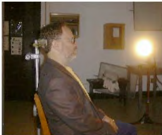
Fig. 6. Converted golf bag cart used as brace for head during 16 exposures.
