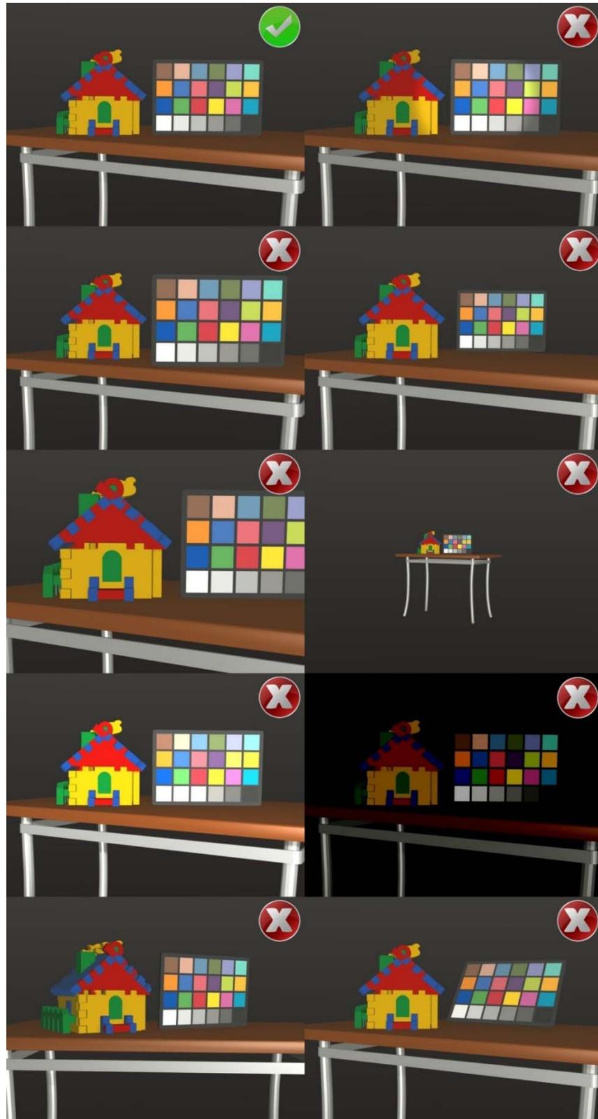
Figure 6: Illustrated photography guidelines. Top row: good image, image with uneven lighting. Second row: chart not in the same region of interest (toy house). Third row: chart not in view, poor framing (too small). Fourth row: over-exposed and under-exposed image. Bottom row: scene not perpendicular to optical axis, and chart is angled.
