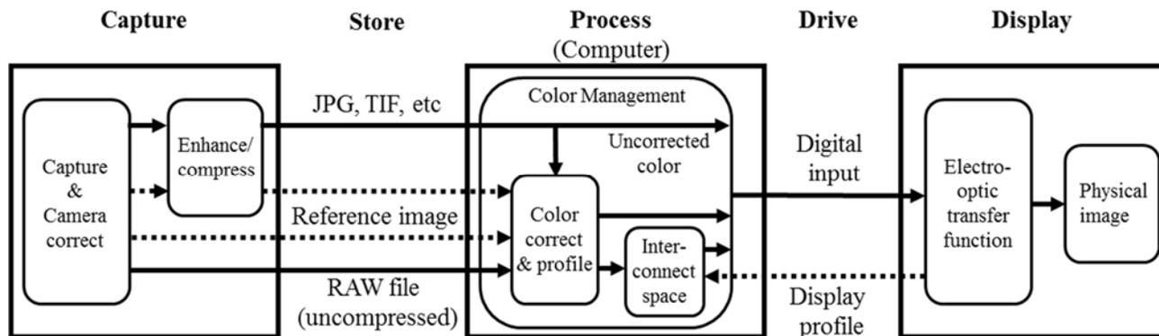
Figure 1: Functional flow diagram of a generic digital color image process, from image capture to its display. The concept of the reference image is used for workflows where color correction is applied.
