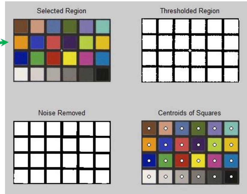
Software was used to crop the area of interest, identify the centroids of each color patch, extract the average RGB and XYZ tristimulus values over 21x21 pixels, then calculate the LAB values of each patch for a D65 white point.
