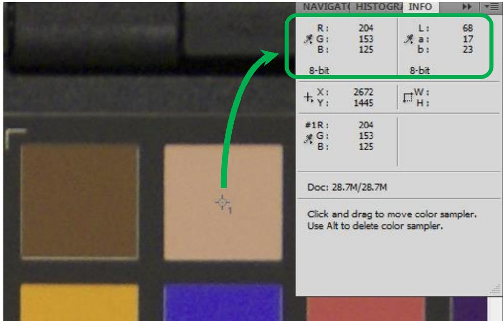
This software calculates the CIELAB values using a D50 white point.
