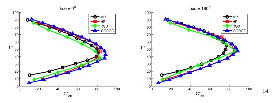
Here Pointer (black curve) and ISORCG (blue curve) gamuts together with real data (read dots and plus) are compared. Generally speaking Pointer gamut is smaller than real data and the ISORCG. However, the two figures show in certain part the Pointer gamut is larger than the ISORCG which is unexpected. Further, some data may be outside the ISORCG as well.
